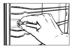
■ Pull on the fastener to release the runner.
